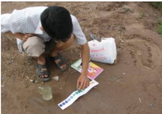
On site pH measurement using test kit
