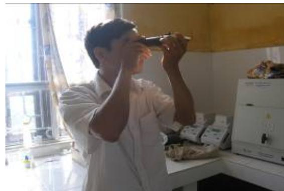
Salinity recordings using refracphoto-metter
