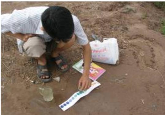
On site pH measurement using test kit
