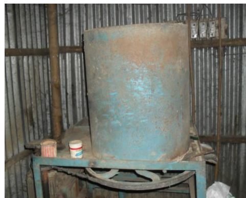
Machine used for mixing hormone with feed
